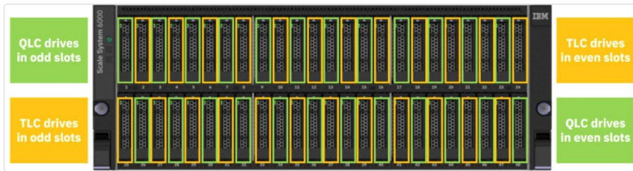
Figure: IBM Storage Scale System 6000 fully populated with 24 TLC and 24 QLC drives
