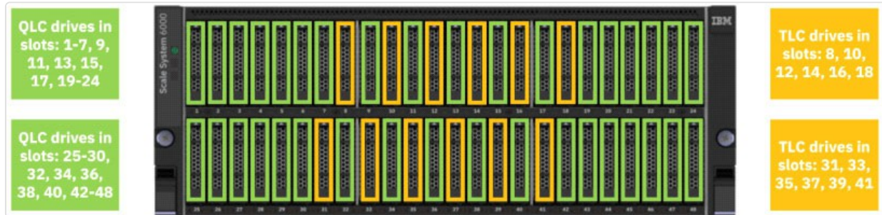
Figure: IBM Storage Scale System 6000 fully populated with 12 TLC and 36 QLC drives
