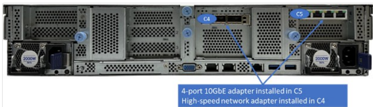
Figure: IBM Storage Scale System single-socket Utility Node EMS adapter layout
