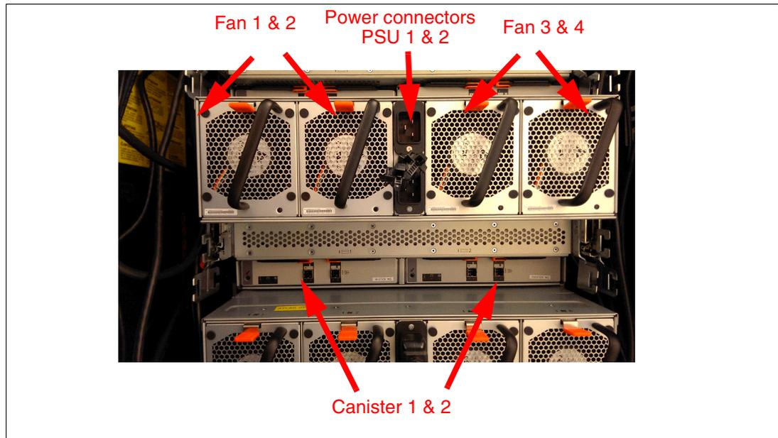
Figure 15 Rear view of IBM FlashSystem 7200 LFF model 92G expansion enclosure
