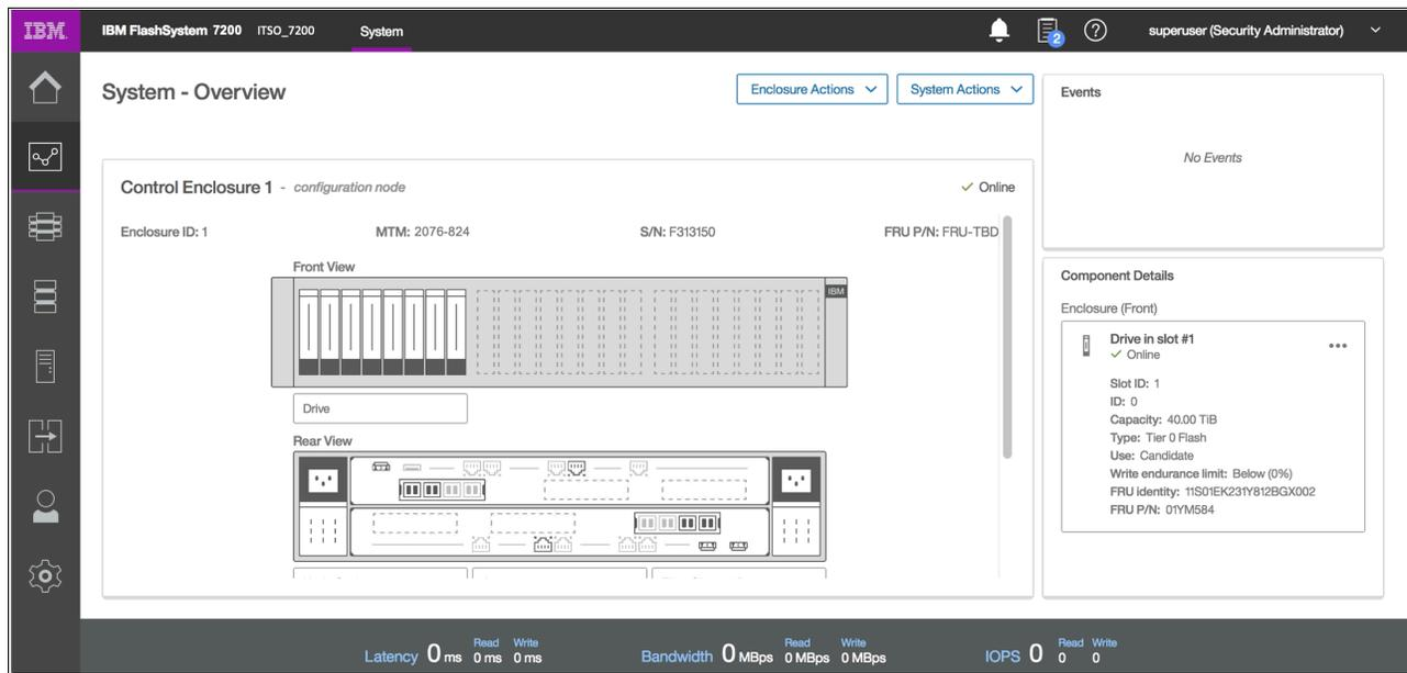
Figure 6 IBM FlashSystem 7200 system overview of the control enclosure
