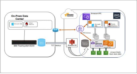
Figure 55 Architecture of backup from IBM FlashSystem 9200 to AWS
