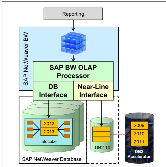
Figure 5 Integration of High-Performance Near-Line Storage in SAP NetWeaver BW
