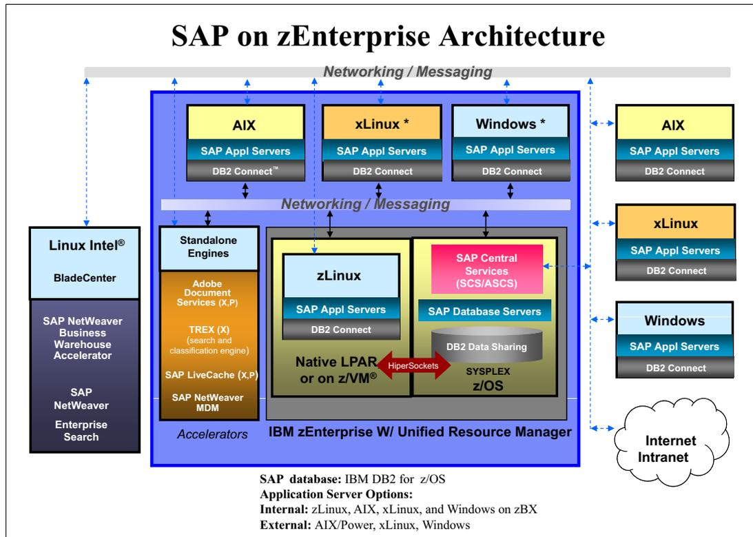
Figure 1 Deployment of SAP on System z
