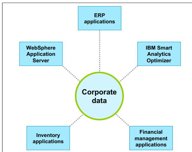
Figure 1 System z hub-and-spoke architecture
