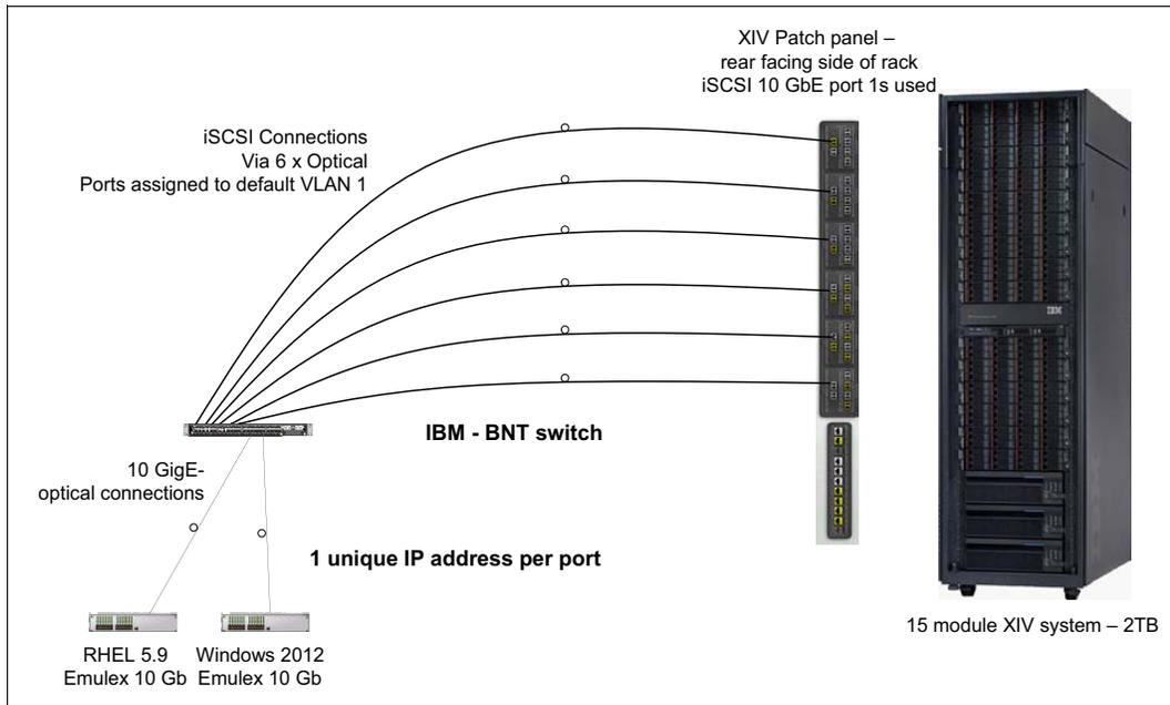
Figure 1 Littleton Lab iSCSI configuration
