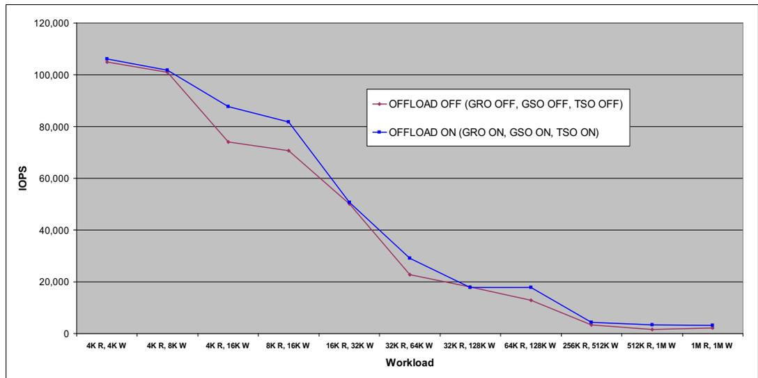
Figure 6 iSCSI results on Linux with and without TCP/IP offload
