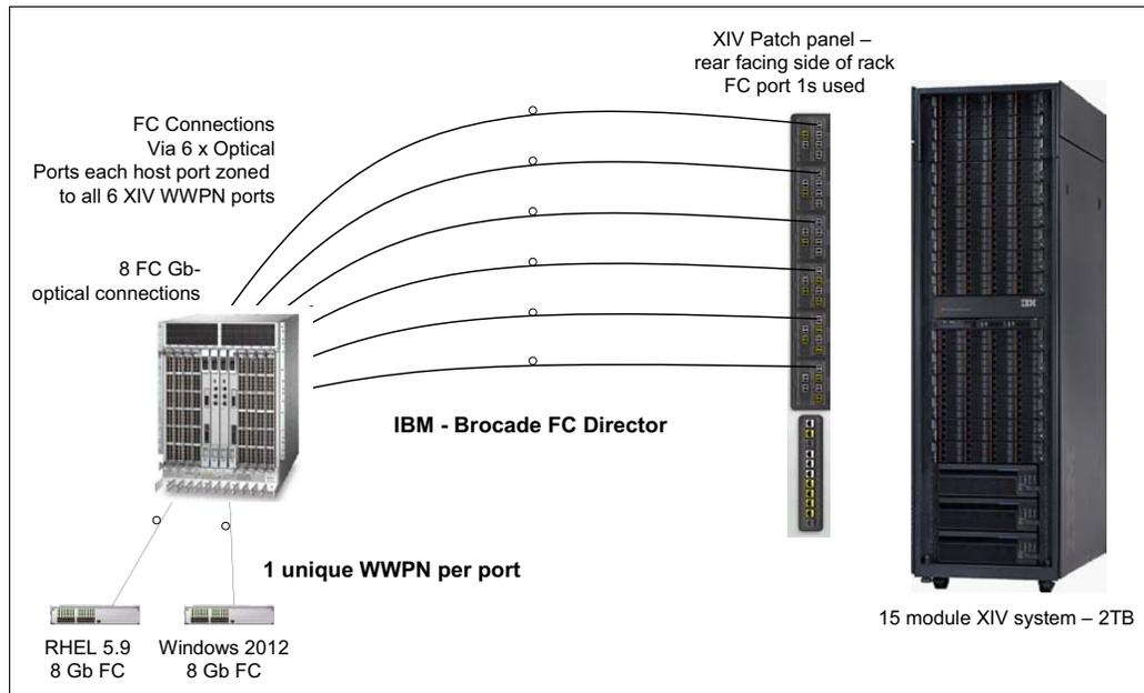
Figure 2 Littleton Lab Fibre Channel configuration
