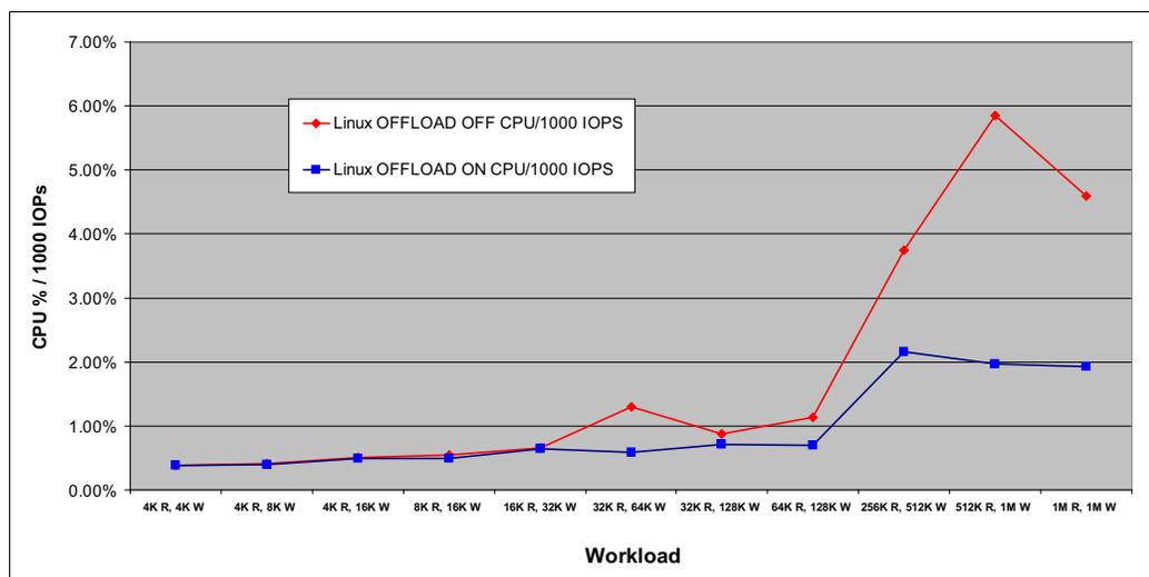
Figure 7 Processor usage with and without offload
