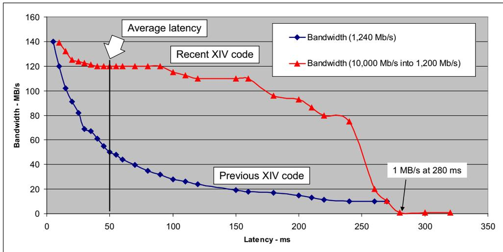
Figure 16 Bandwidth to latency comparison between version of the XIV code (storage software)
