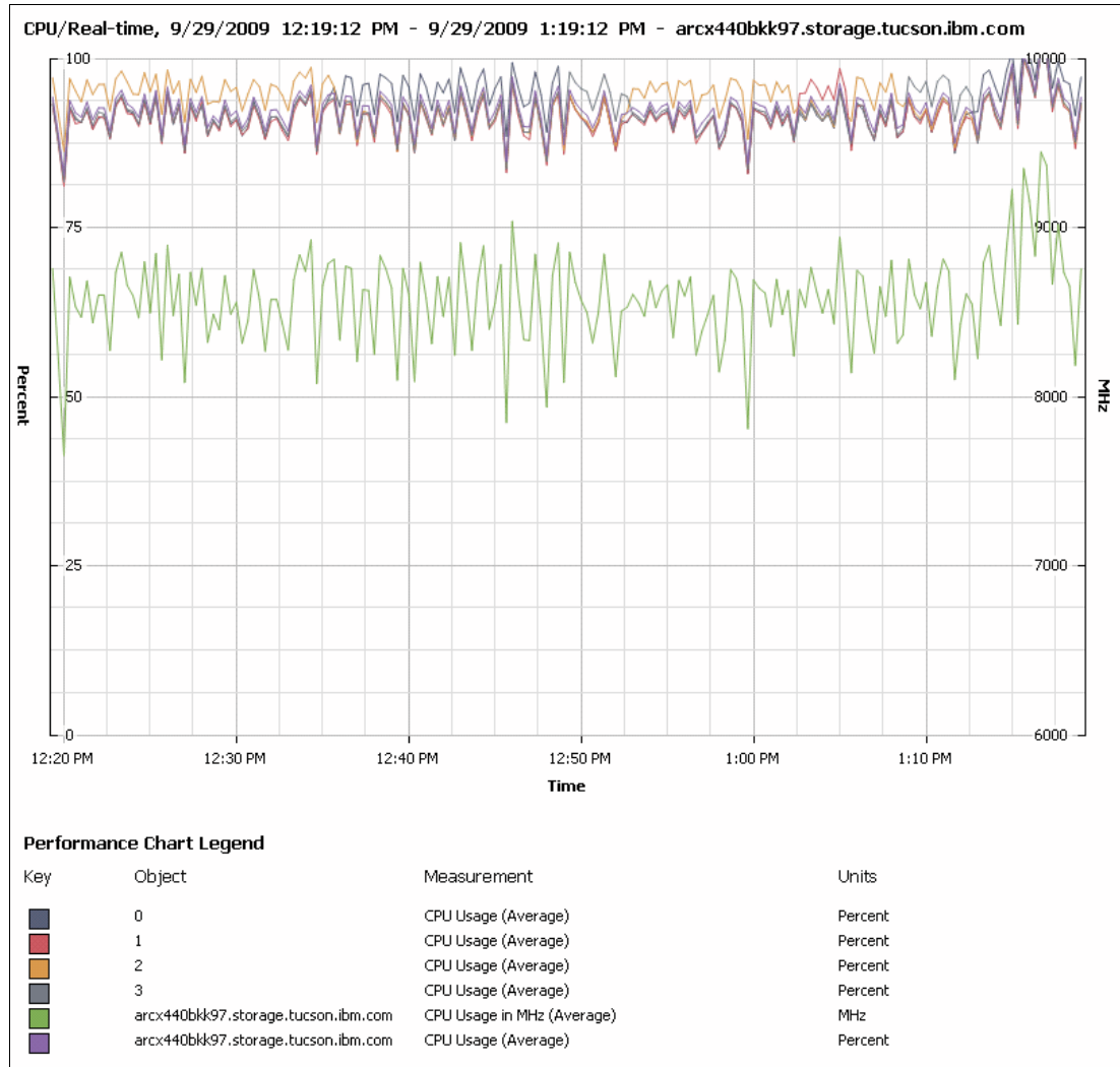
Figure 28 Single ESX host CPU load during performance testing
