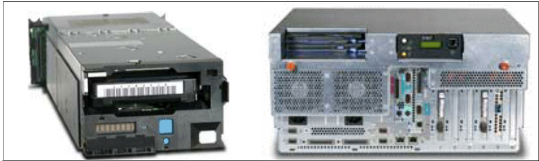
Figure 3 3592 J1A tape drive and 3592 J70 controller
