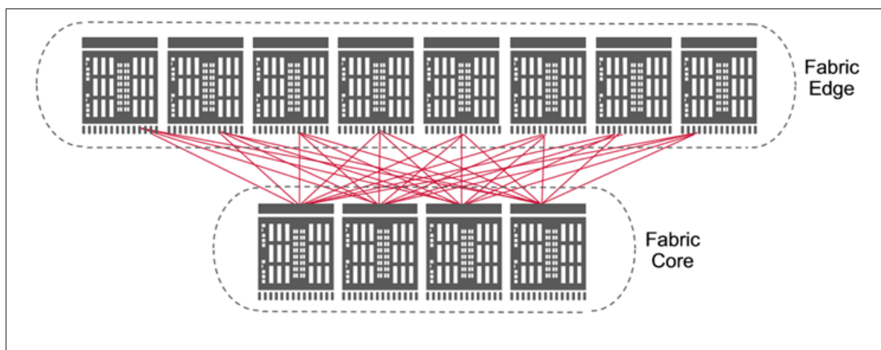
Figure 5-4 A 12-chassis UltraScale ICL-based core-edge design
