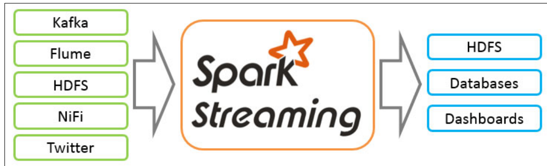
Figure 5-5 Flow of the Spark Streaming engine
