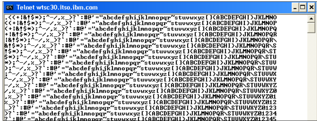
Figure 6-5 Verifying the chargen service
