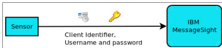
Figure 4-4 An MQTT client authenticating with a client ID, user name, and password
