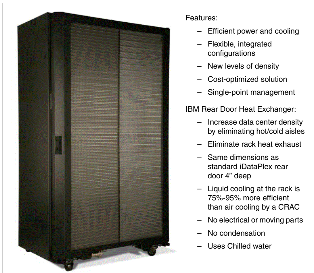
Figure 2-22 IBM System x iDataPlex with Rear Door Heat Exchanger
