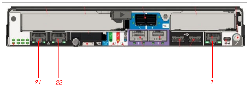
Figure 5-1 ProtecTIER network interfaces for customer and replication network on Gateway model
