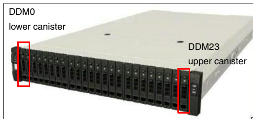
Figure A-3 DD6 server front view and pt_work partition location based on canister that mounts it
