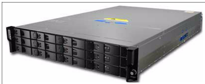
Figure 1-2 IBM System Storage TS7620 ProtecTIER Deduplication Appliance Express
