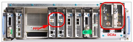
Figure 2-6 Location of PPS ports (first processor drawer)
